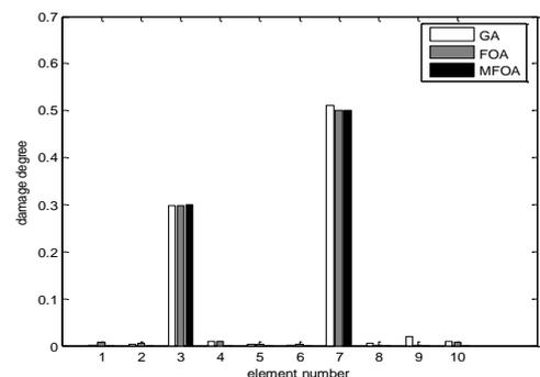
FIGURE 4 Comparison of identification results of multi-damage
