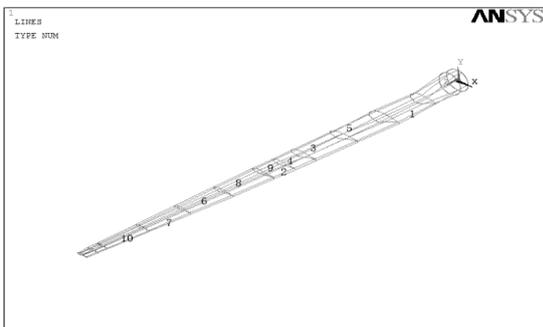
FIGURE 1 Structural model of wind turbine blade
