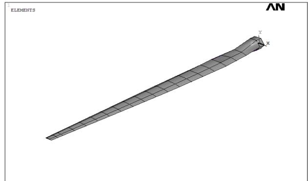
FIGURE 2 Finite element model of wind turbine blade
