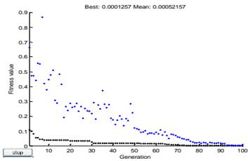
FIGURE 5 Convergence curve for identification of single damage by GA
